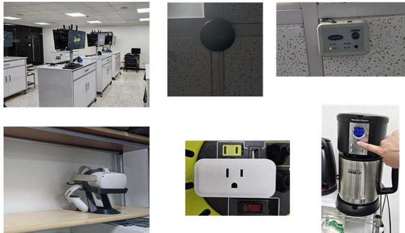
**Figure 1. Devices integrated for the digital twin (Real model). On top of the image are the devices to control the IR signals and temperature/humidity reads. On the bottom side, is the devices to control the power reads.**
